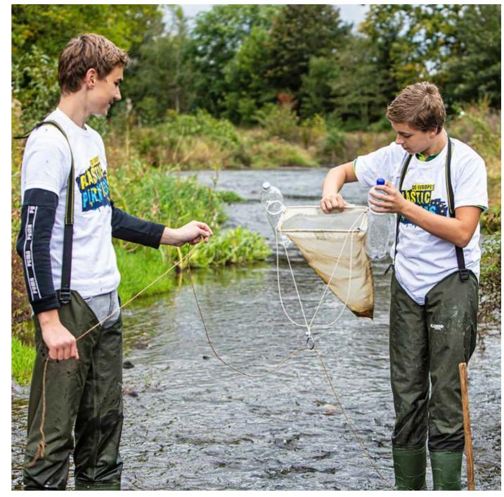
In full gear: participants in the campaign prepare to test the river for microplastics. To ensure that the data collected is comparable, the standardised special net is provided by the campaign. Photo: BMBF/Gesine Born
